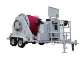
10,000lb class drum puller with 1" pulling rope featuring a John Deere diesel engine, hydraulic drive, with manual levelwind. Fast and efficient puller without requiring the need for an additional reel carrier for the pulling line.
