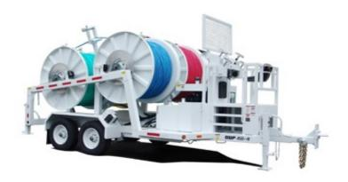
The ODP 40-4 is a four drum puller capable of line pull of 4,000 lbs on a single drum. Each drum can be engaged or disengaed for single or multiple drum pulling. An overspin brake with a hydraulic actuator is also included on each drum. Operator controlled post style levelwind allows for even winding of rope.
